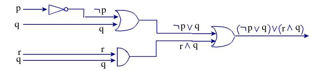
2. Determine the output of the combinatorial circuit:
